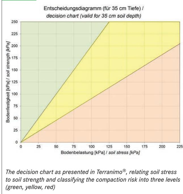
The border between the green and yellow hazard levels corresponds to a soil stress equal to 50 % of the soil strength. According to the current level of knowledge, this border represents the transition of a soil from completely elastic behaviour to initial plastic deformation of the soil structure: Keller et al. [15] were able to show that a direct transfer of precompression values obtained from laboratory oedometer readings to the strength of soils in the field is not possible.
