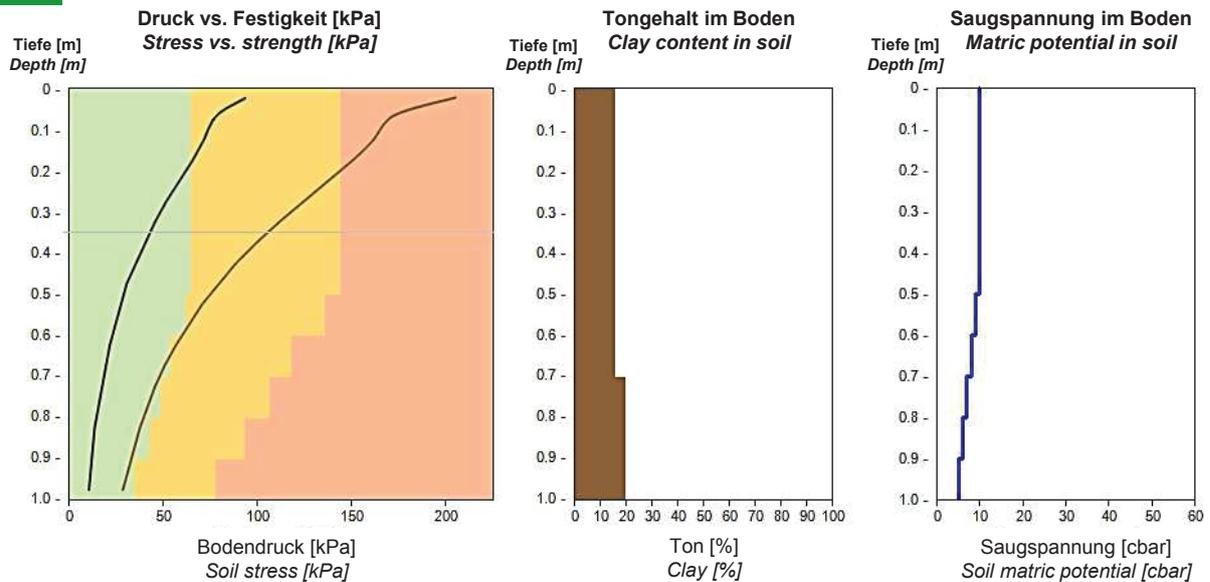
Result plots in Terranimo<sup>®</sup> expert. Left: soil stress under two different wheels (lines) and soil strength (green, yellow, red) in the soil profile. Middle and right: corresponding clay content, and soil matric potential
