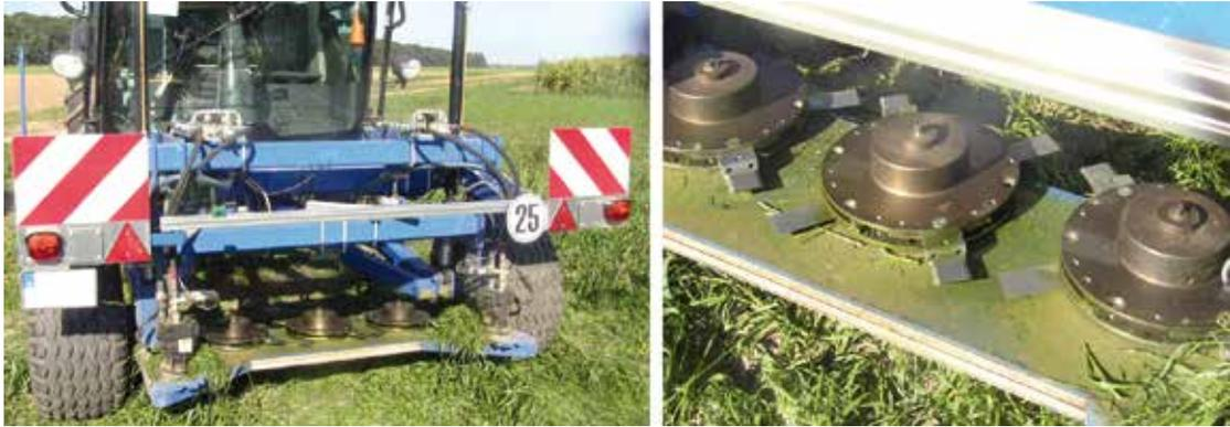
Test machine with functional prototype mower (left) and mower bar with cutting units "2/2" (right) (Photos: S. Kemper)
