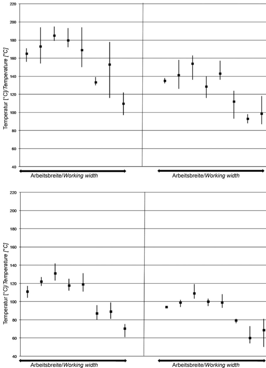
Maximum temperatures (arithmetic mean and span) across the working width (850 mm) of the thermal weed control device at working speed of 0.35 m/s (top left), 0.42 m/s (top right), 0.53 m/s (down left) and 0.81 m/s (down right), ( $n = 3$ )
