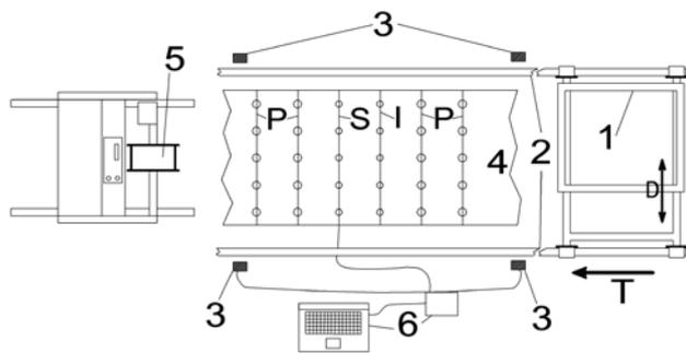
Sketch of test bench with: 1 waggon with top slide, 2 rails, 3 photoelectric relays, 4 target surface with holes for thermocouples (S), model plants (P) and indicators (I), 5 winch, 6 device for data sampling and data storage, T direction of travel, D direction of displacement
