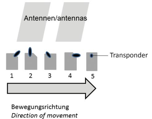
Orientation of the tags on the platform regarding to the direction of movement
