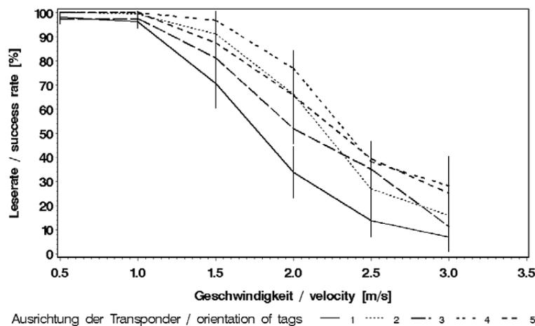
Success rate of registration depending on orientation of the tags on the platform and the velocity during the test
