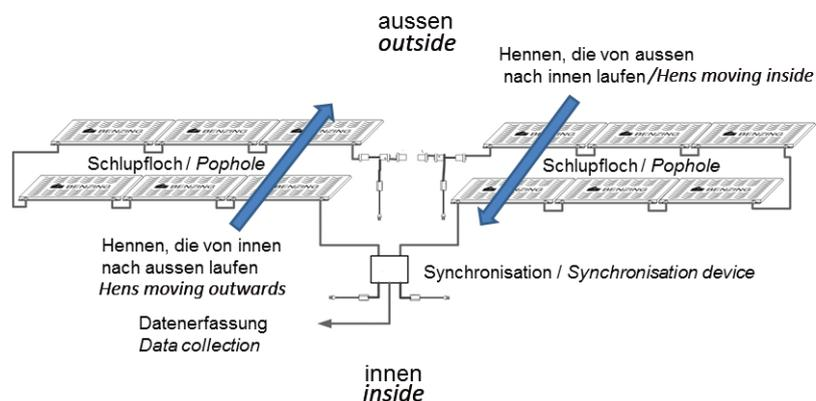
Set-up of the RFID system at two popholes during the on-farm application
