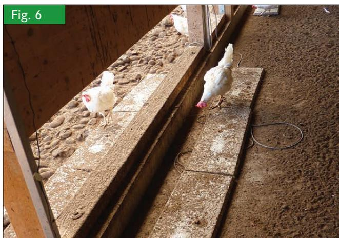
RFID antennas on both sides of a pophole during the field test (Photo: S. Gebhardt-Henrich)
