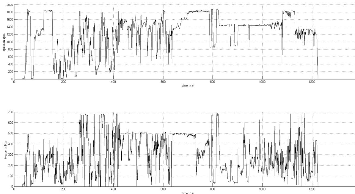
Figure 12: Dynamic load cycle to validate the thermal simulation model
