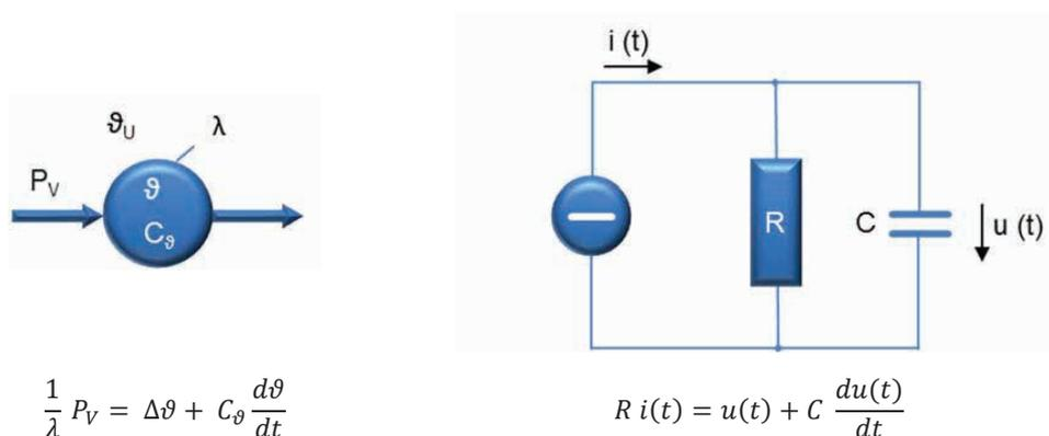
Figure 4: Analogy of a heat source network and an electric network
