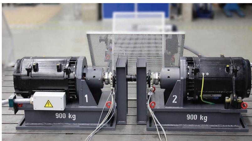
Figure 10: Mechanically coupled engines for parameter identification (photo: C. Pohlandt)
