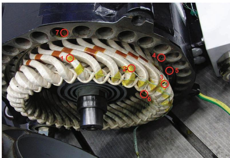
Figure 9: Temperature measuring points at stator winding for measurements of temperature profiles (photo: C. Pohlandt)
