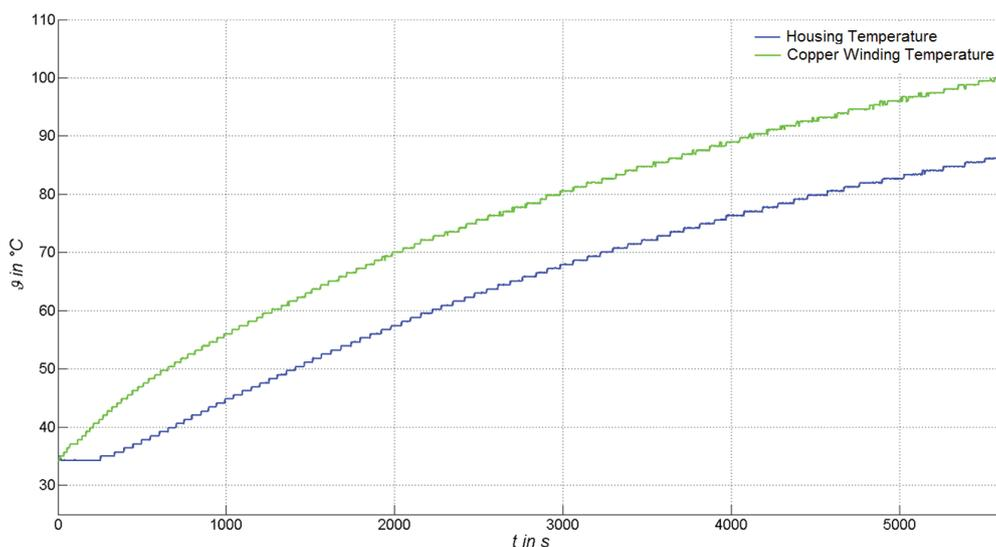
Figure 7: Simulated curves of initial temperature gradient of copper winding and housing
