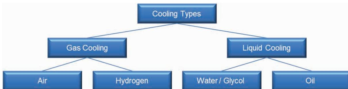
Figure 2: Coolant types of electric machines
