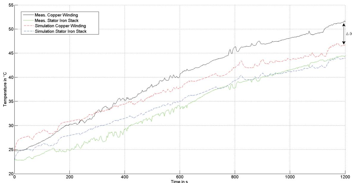
Figure 13: Comparison of the temperature profiles between simulation and measurement under dynamic workload
