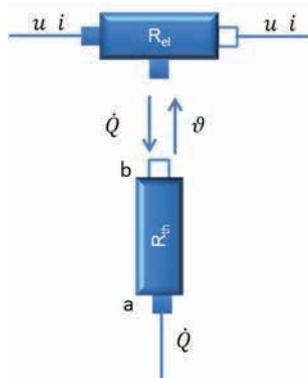
Figure 5: Model of a thermal and electrical resistance with bidirectional data flow
