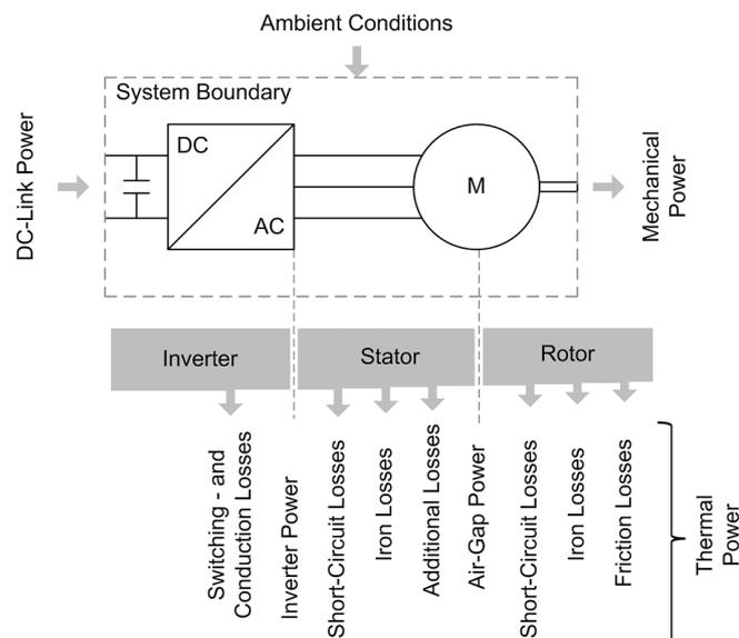
Figure 1: System boundary of the electric powertrain including assigned losses
