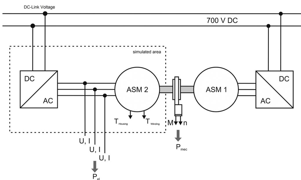
Figure 11: Schematic experimental setup to validate the simulation model under dynamic workload
