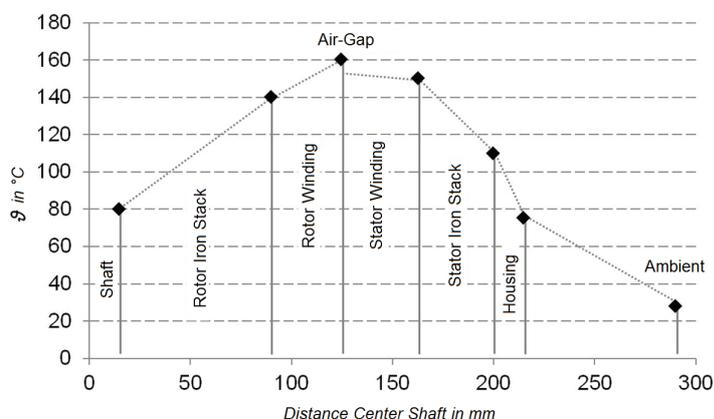
Figure 8: Stationary temperature distribution from the shaft centre simulated in steady state conditions
