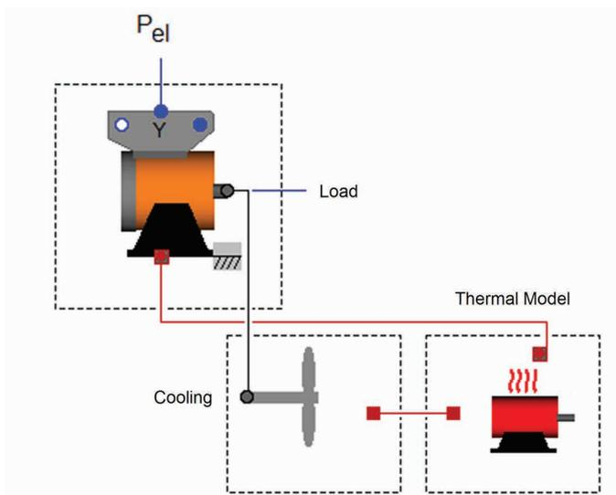
Figure 6: Noncausal simulation model of a self-cooled asynchronous machine
