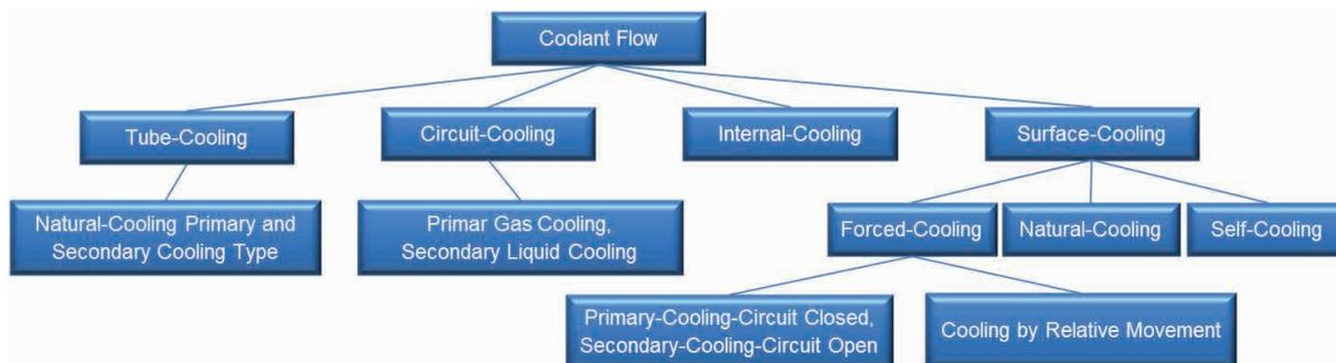
Figure 3: Coolant flow in electric machines
