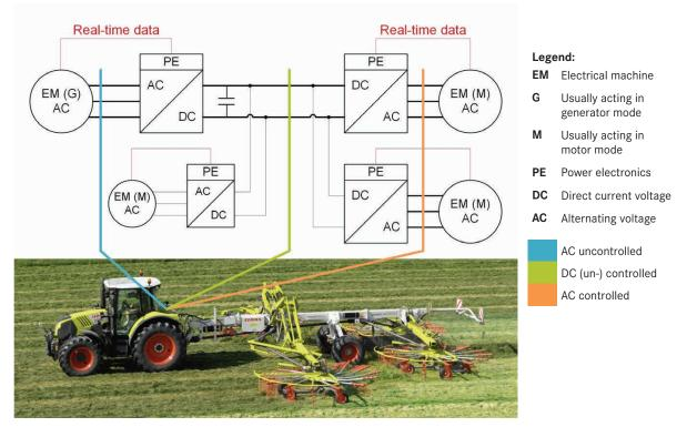
Figure 1: Basic structure and potential solutions for interface of an electric drive system
