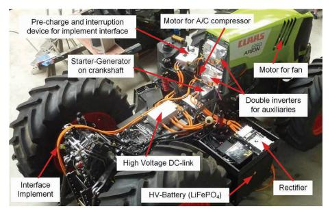
Figure 3: High Voltage system in the CLAAS Arion 650 Hybrid (cooling not shown)
