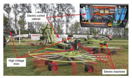
Figure 5: Function model CLAAS E-Liner 4000
