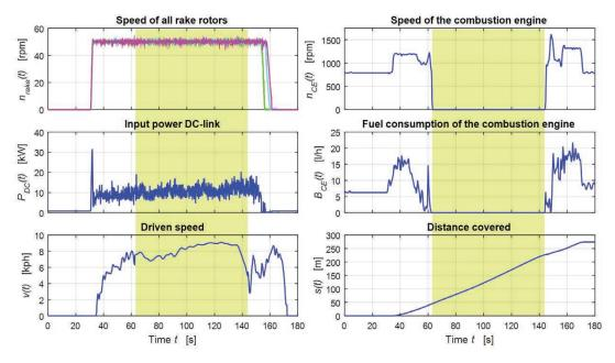
Figure 4: Emission-free use of the swather (green indication) in the used SOC region (25 %)
