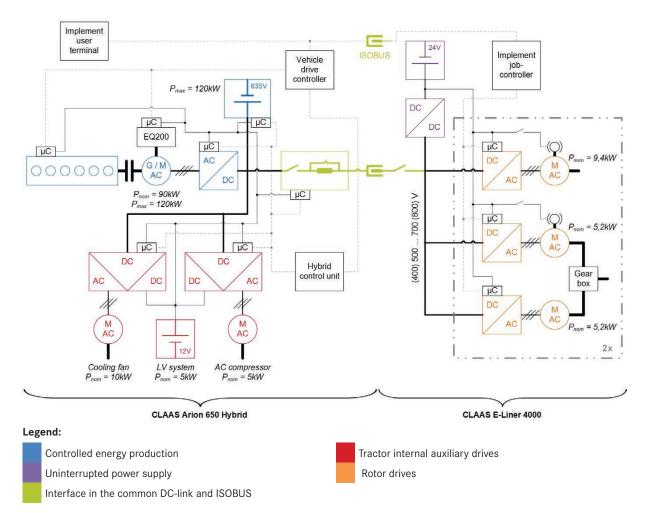
Figure 2: Block diagram of the total architecture of the electric system of the functional models
