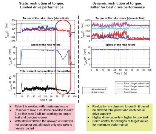
Figure 7: Explanation of the dynamic load management using the example of two rotors of the swather
