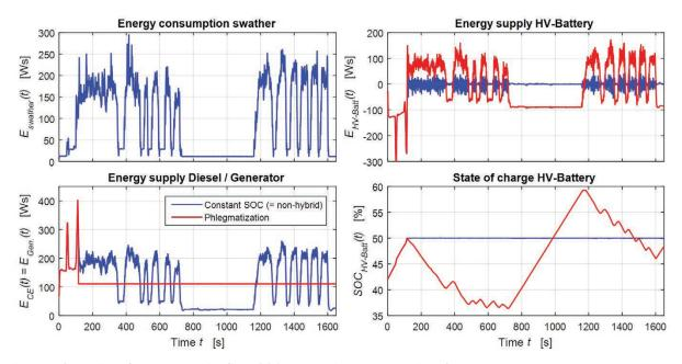
Figure 8: Operating of the tractor with fixed SOC and hybrid strategy derived from that
