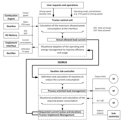
Figure 6: System-wide approach for load limitation and load prediction
