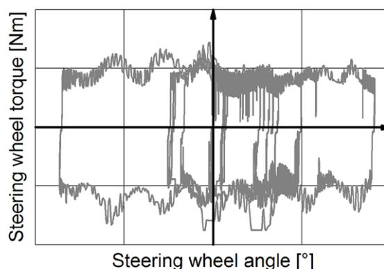
Figure 3: Characteristic of a fully hydraulic steering system
