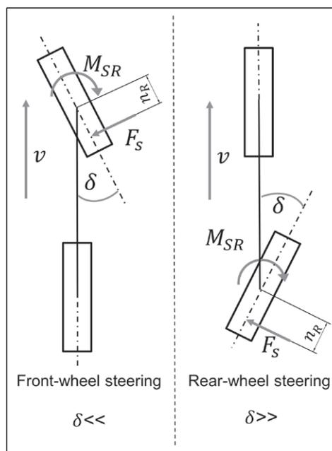
Figure 2: Tire aligning torque of a front-steered and a rear-steered vehicle
