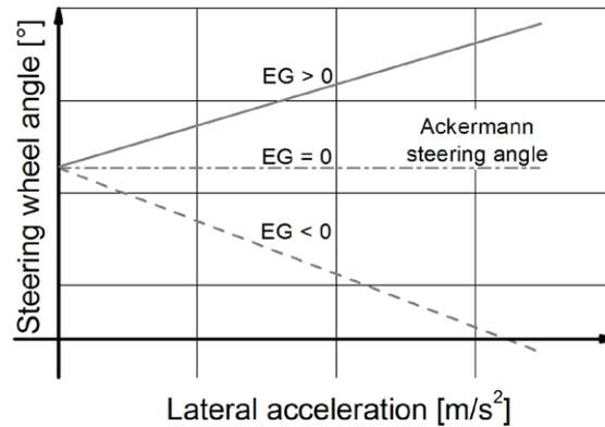
Figure 1: Required steering wheel angle at constant path radius according to SCHINDLER (2007)
