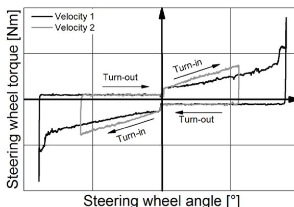
Figure 5: Steering torque curve of the SbW system
