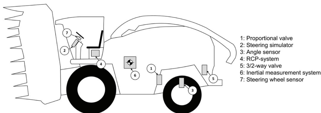
Figure 4: Schematic arrangement of the components in the test vehicle
