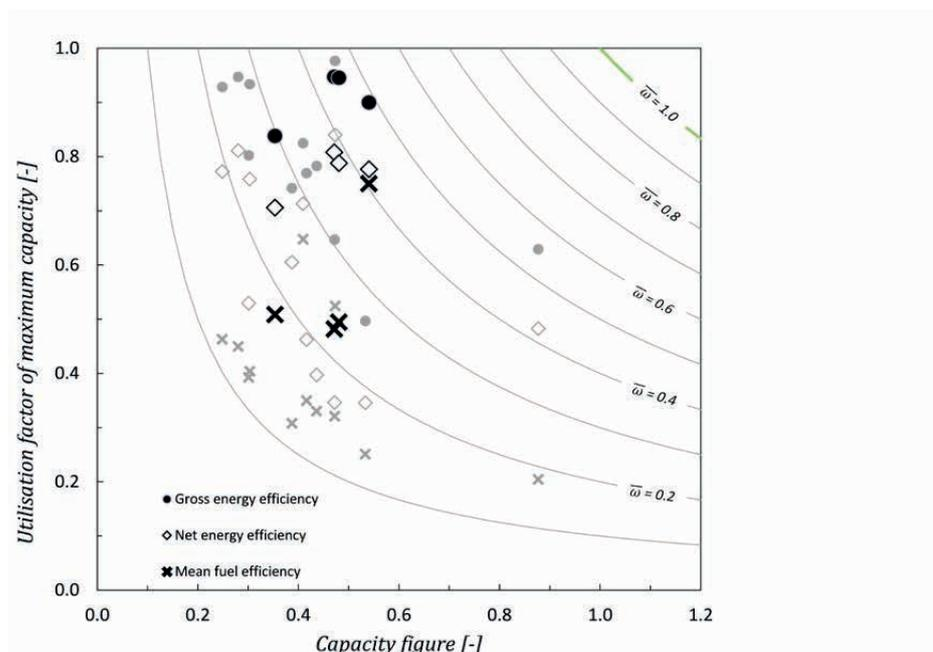
Figure 5: Mean fuel efficiencies of the four agricultural biogas plants studied (black) compared to similar biogas plants from Biogas Measuring Programmes 1 and 2 (grey) (FACHAGENTUR NACHWACHSENDE ROHSTOFFE E.V. 2005, 2009).
