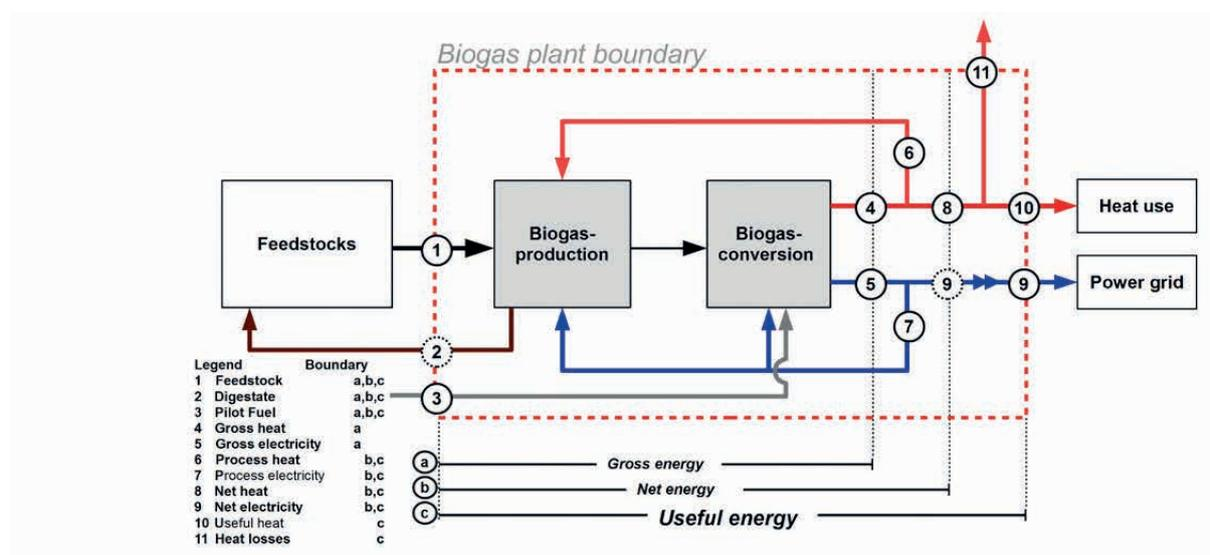
Figure 1: The assessment boundaries of the biogas process for assessing the gross, net and useful energy.
