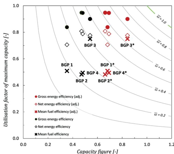
Figure 6: Mean fuel efficiencies of the four plants in our study without (black) and with (red) adjustment of the gross calorific value for the fermentable organic matter (FOM)
