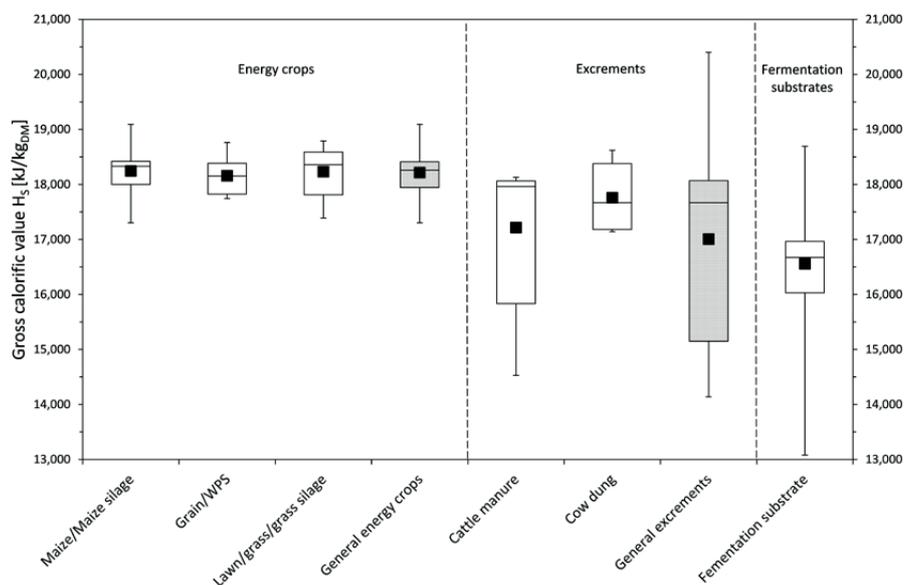
Figure 4: Ranges of variation, median values (line in the box), and averages (black dot) of the gross calorific values of dry matter.
