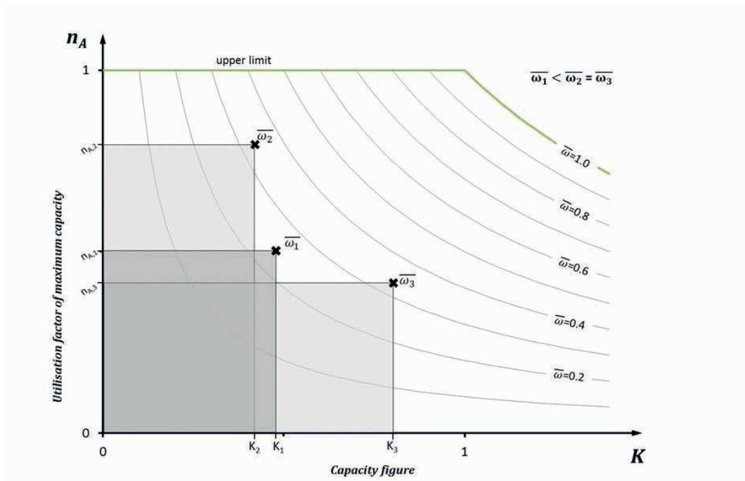
Figure 3: Scheme of the mean fuel efficiency of different plants and/or comparison of one plant over multiple years
