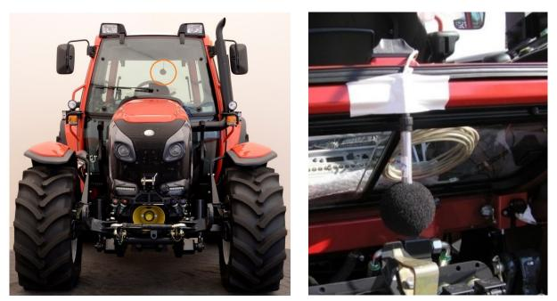
Figure 3: Microphone position (airborne sound microphone driver, airborne sound microphone near field transmission rear) on the Lintrac 90 (Photo: Lindner Traktorenwerk GmbH)
