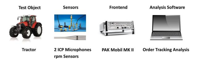
Figure 1: Measurement chain
