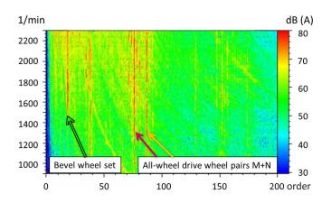
visible red lines of the bevel wheel sets and the all-wheel drive wheel pairs, resonances are also recognisable as hyperbolas.
