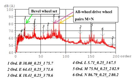
Figure 6: Geotrac recording, order tracking analysis of airborne noise in near field transmission rear
