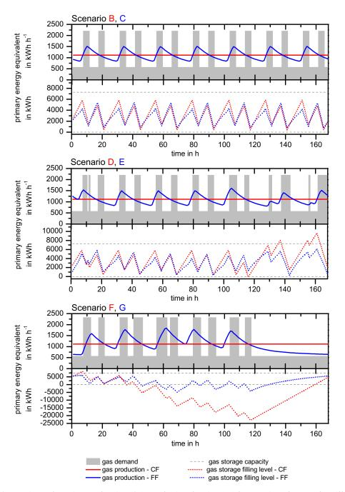
Figure 8: Comparison of continuous feeding (CF) and flexible feeding (FF) for a period of 7 days for different scenarios. Course for gas demand, gas production and gas storage filling level for scenario B vs. C; scenario D vs. E and scenario F vs. G
