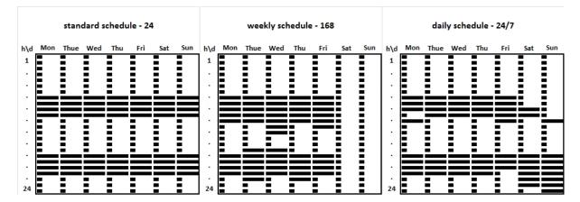
Figure 4: Matrices for one week showing the relative power feed in, 24 rows (h) by 7 columns (d), of 3 schedules (standard schedule, daily schedule, weekly schedule), the shorter bars representing the continuously running combined heat and power unit (CHP-unit, CHP) with 250 kW, the larger bars shows an operating state, where in addition the CHP with 750 kW is in operation
