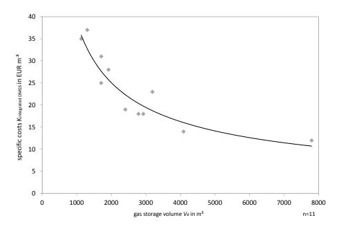
Figure 7: Specific costs of integrated double membrane gas storage on top of the fermenter (n=11)
