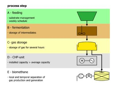
Figure 1: Approaches for a flexible operation of a biogas plant referring to the process chain, source: own diagram, based on ORTWEIN et al. (2014)
