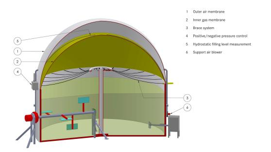
Figure 6: Structure continuous stirred-tank reactor (CSTR) with integrated double membrane gas storage, source: adapted from (Liebetrau et al. 2015)
