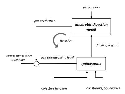
Figure 5: Schematic description of the model-based optimisation of gas production according a power generation schedule
