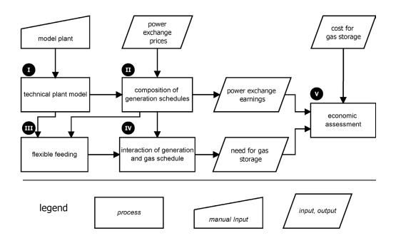
Figure 3: Block diagram of model components (mapped as rectangle processes) for evaluation of flexible feeding
