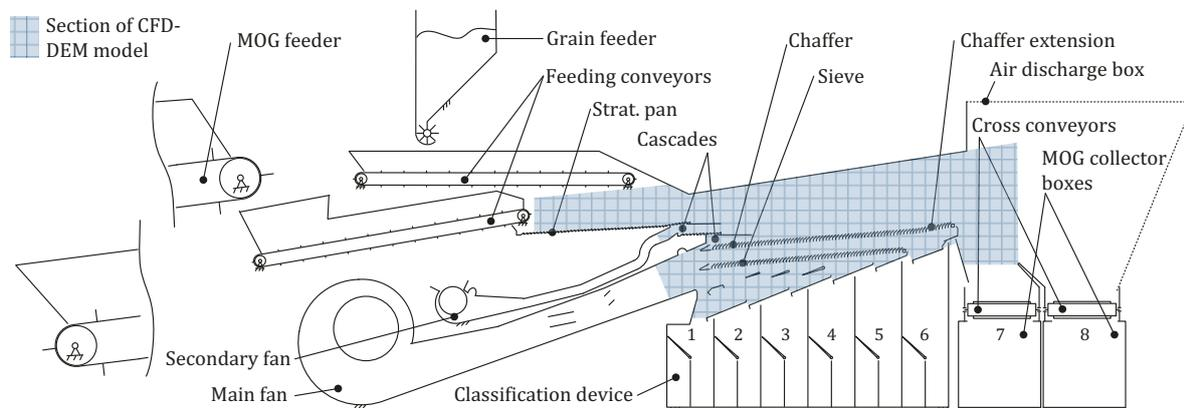
Figure 7: Design of experimental cleaning device test rig and indication of section of CFD-DEM model
