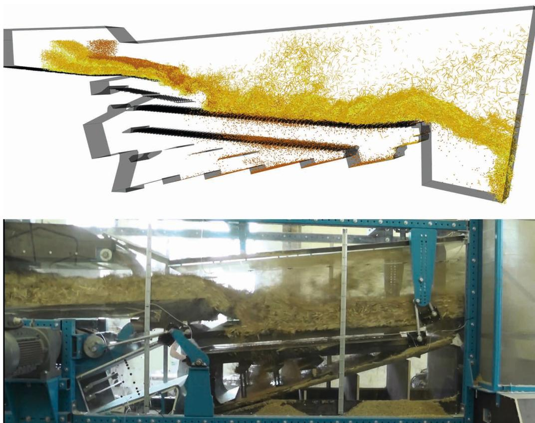
Figure 8: Snapshots of numerical separation (upper picture) and experimental separation (lower picture) in a combine cleaning device segment at stationary period for rel. MOG feedrate of 2.38 kg/(s m)
