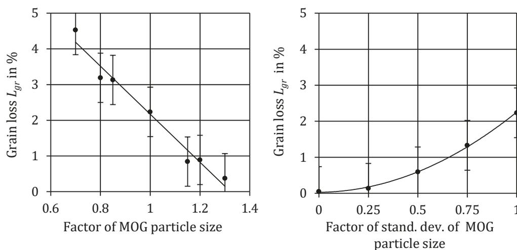
Figure 5: Results of simulation – left: grain loss as affected by factor of MOG particle size, right: grain loss as affected by factor of standard deviation of MOG particle size, (MOG feedrate  $q_{\text{MOG}} = 1.79 \text{ kg}/(\text{s m})$ , Factor of fluid velocity at main inlet  $\text{FFV}_{\text{main}} = 1$ )
