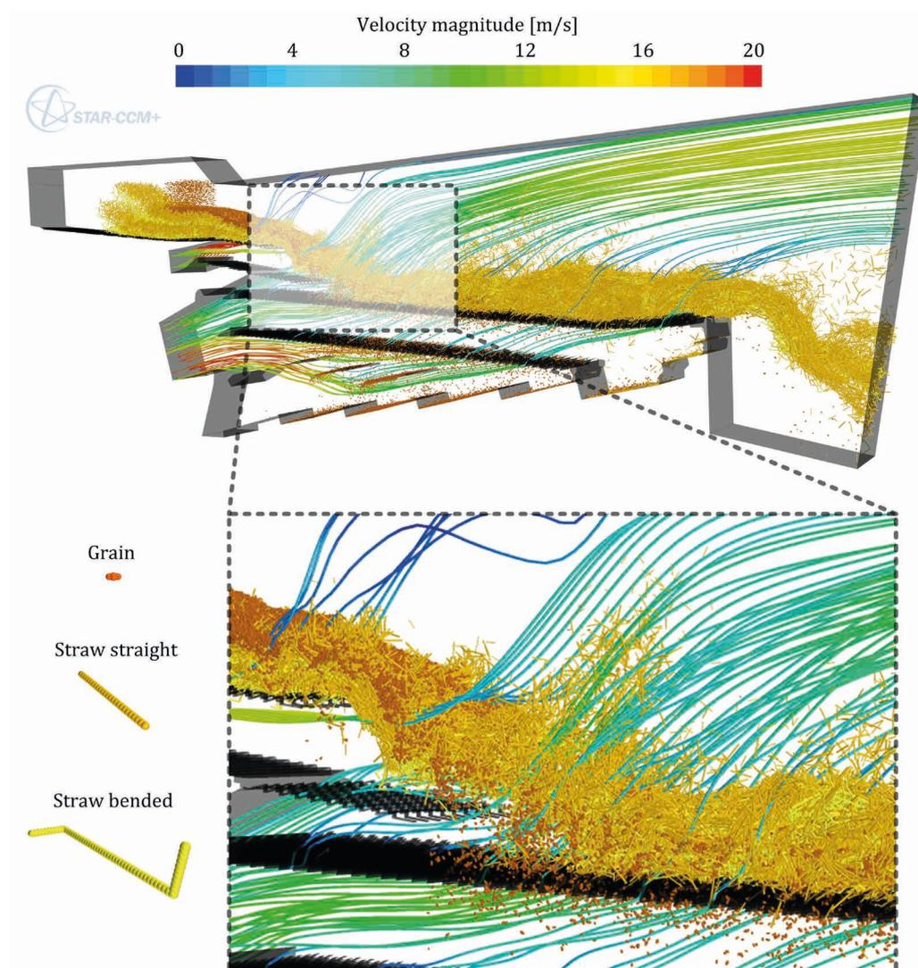
Figure 4: Exemplary graphical representation of results: DEM particles (particle legend not in scale) and streamlines (colored by fluid velocity)
