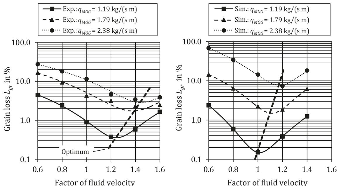
Figure 9: Interaction of relative MOG feedrate and fluid velocity at main inlet on grain loss; comparison of experimental results (left) and numerical results (right); factor of fluid velocity represents a factor multiplied to nominal fan turning speed
