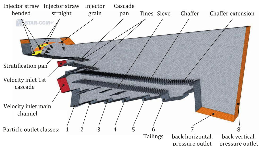
Figure 3: CFD-DEM model of cleaning device segment
