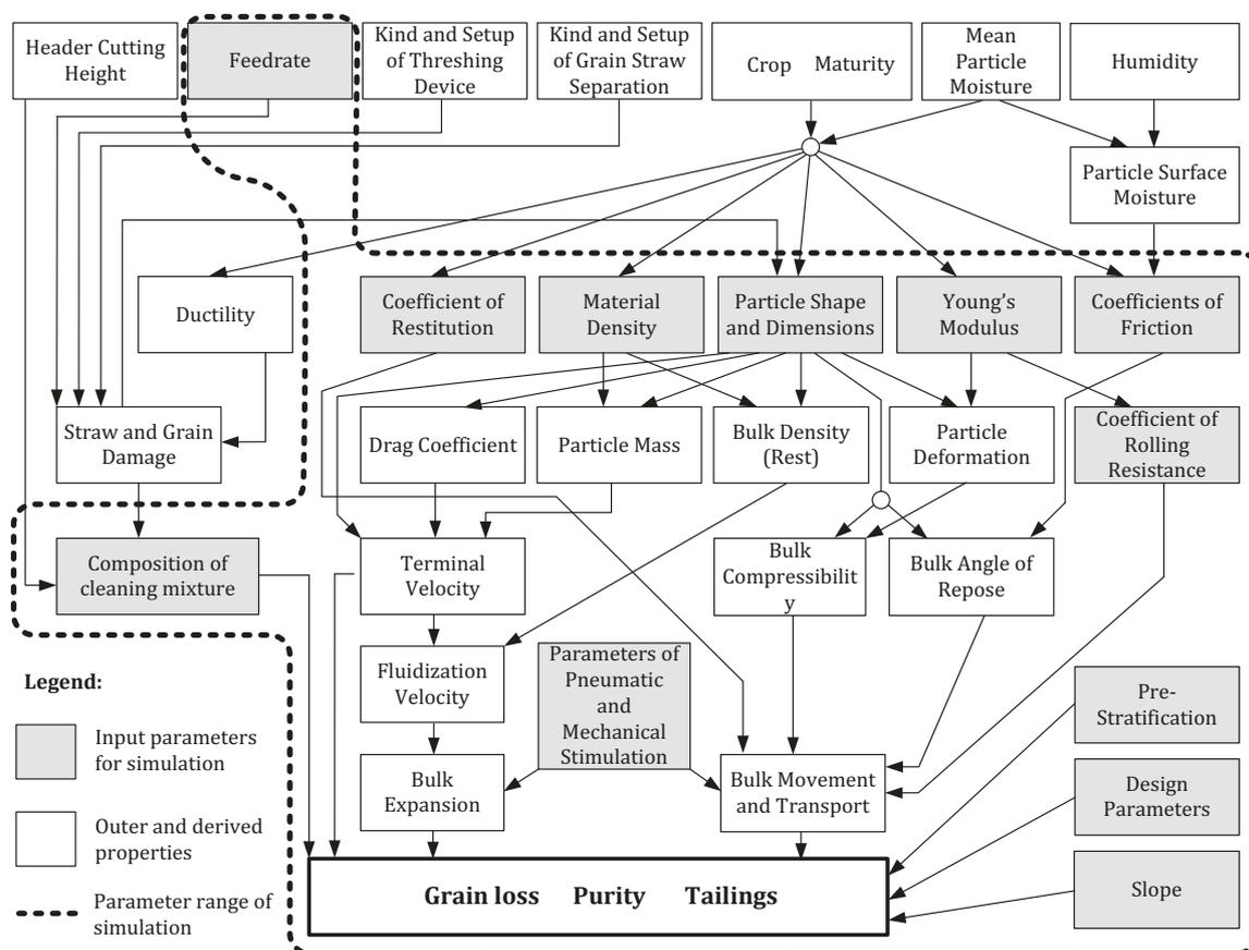
Figure 1: Correlation between target values (grain loss, purity and tailings) and process factors (ambient conditions, particle properties, etc.) of separation process; identification of direct input parameters of the simulation
