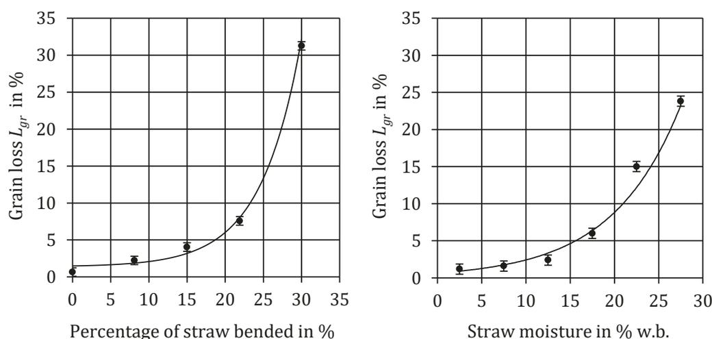
Figure 6: Results of simulation – left: grain loss as affected by mass percentage of bended straw, right: grain loss as affected by straw moisture (MOG feedrate  $q_{\text{MOG}} = 1.79 \text{ kg}/(\text{s m})$ , Factor of fluid velocity at main inlet  $\text{FFV}_{\text{main}} = 1$ )
