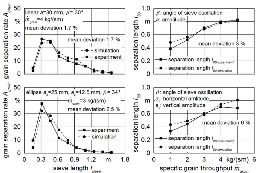
Figure 9: Comparison of the grain separation rate  $A_{grain}$  and the grain separation length  $l_{80}$  of simulation and experiment for linear (BECKMANN et al. 2016) and elliptical sieve movements
