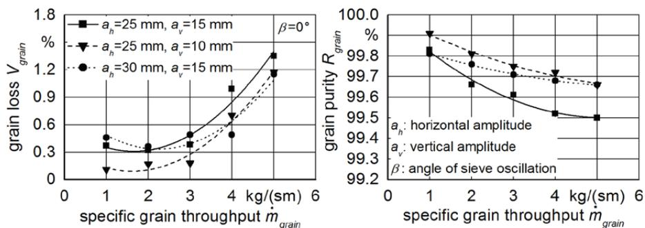
Figure 7: Comparison of the elliptical sieve movement with different parameter sets
