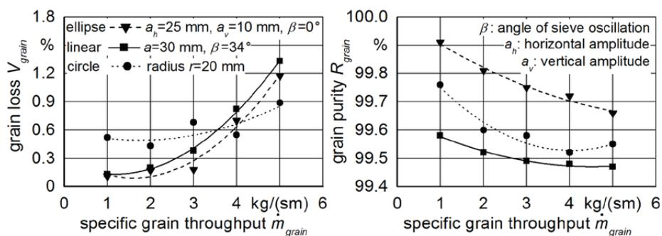
Figure 8: Comparison of the elliptical, circular and linear sieve movements
