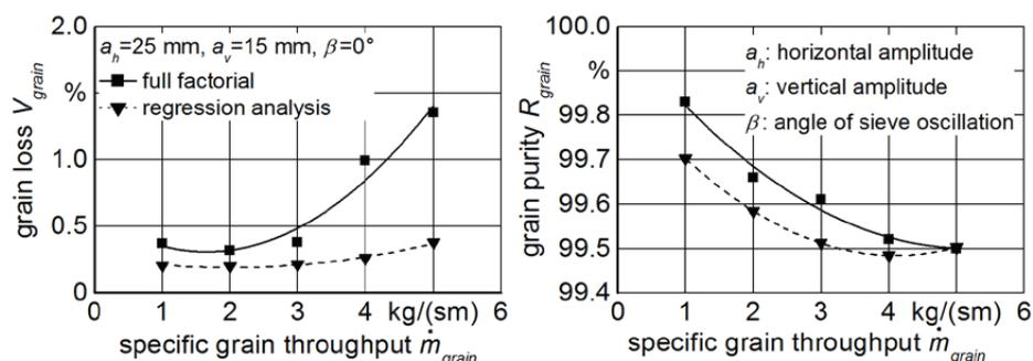
Figure 6: Comparison of grain loss and grain purity of a full factorial experimental series with the results from the regression analysis with a quadratic regression approach
