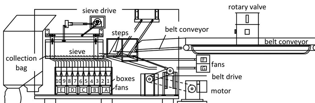
Figure 2: Combine cleaning unit test rig to investigate linear, circular and elliptical sieve movements (BECKMANN et al. 2016)
