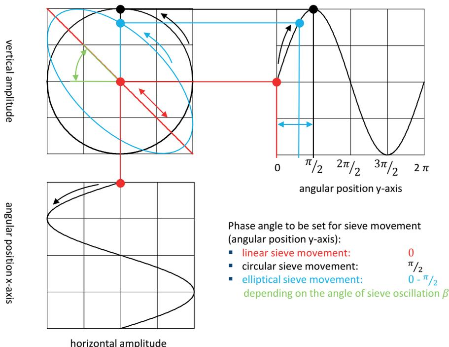
Figure 4: Adjustment of the linear (red), circular (black) and elliptical (blue) sieve movement with the phase angle, angle setting horizontal und vertical axis in radians
