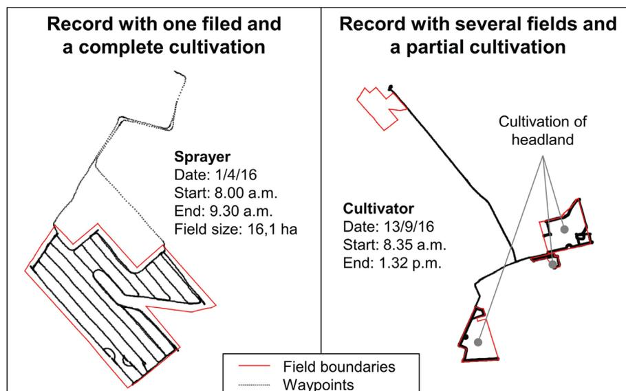
Figure 5: Fields and recorded tracks (waypoints); left: record with cultivation of a field including headland; right: record with cultivation only of headland of 3 fields
