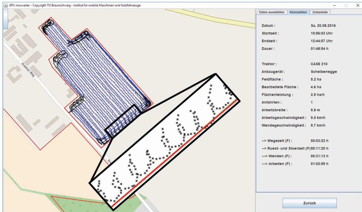
Figure 6: Screenshot of evaluation program with a selected process step of stubble cultivation with a disc harrow; calculated key values and visualization of the suboperations (working (blue) and turning (black, enlarged) in the field)
