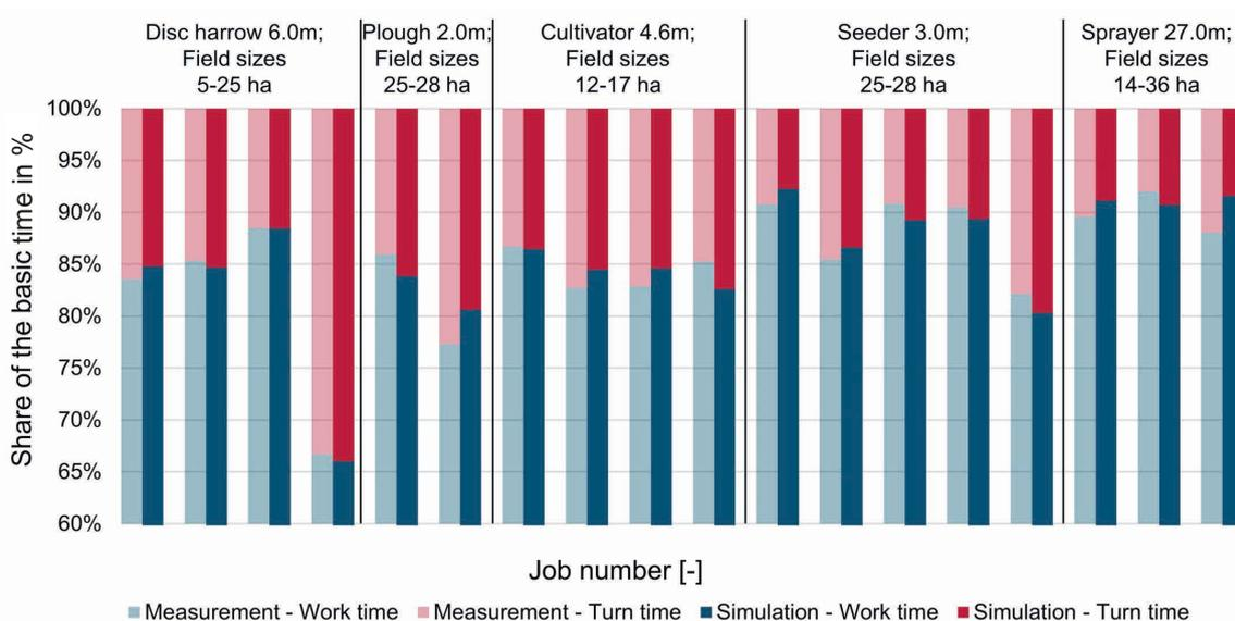
Figure 7: Results from simulation and measurement for different jobs and implements
