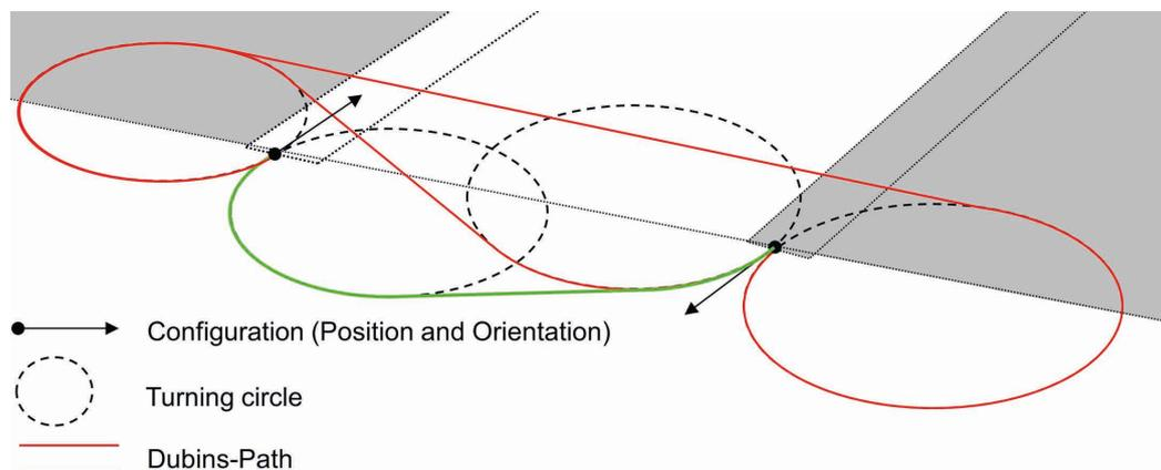
Figure 3: Dubins path with configuration of start- and endpoint using example of a turning manoeuvre in headland
