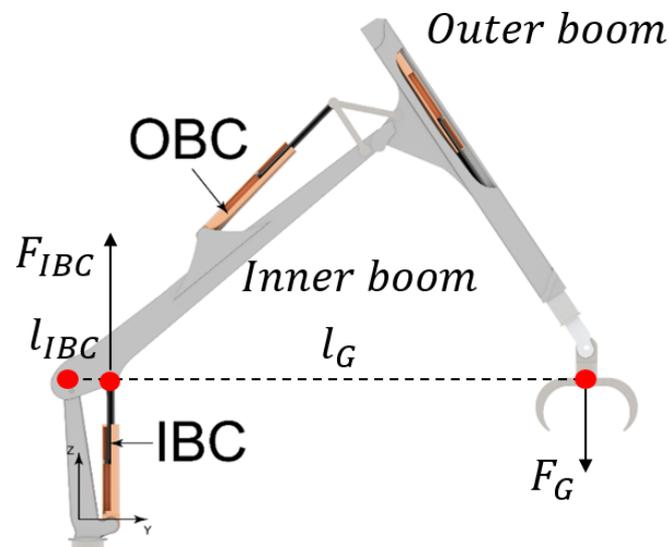
Figure 1: Force application position at a forestry crane
