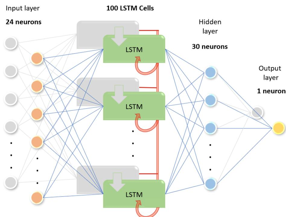
Figure 4: Used network structure including LSTM cells
