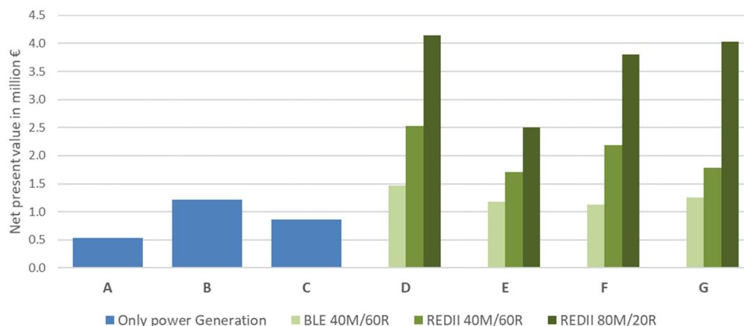
Figure 8: Comparison of the overall profitability of the seven connection scenarios for a 500 kW<sub>el,inst</sub> BGA – scenarios A to C with electricity generation only, D to F with proportional electricity and fuel production and G with complete fuel production
