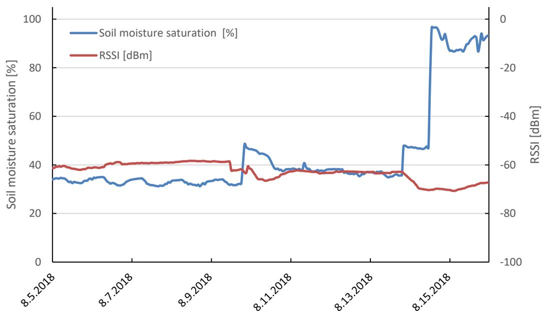
Figure 5: Influence of soil moisture saturation on the RSSI. The indicator decreases when the amount of water in the soil increases, such as on rainy days (August 9th and August 13th/14th).
