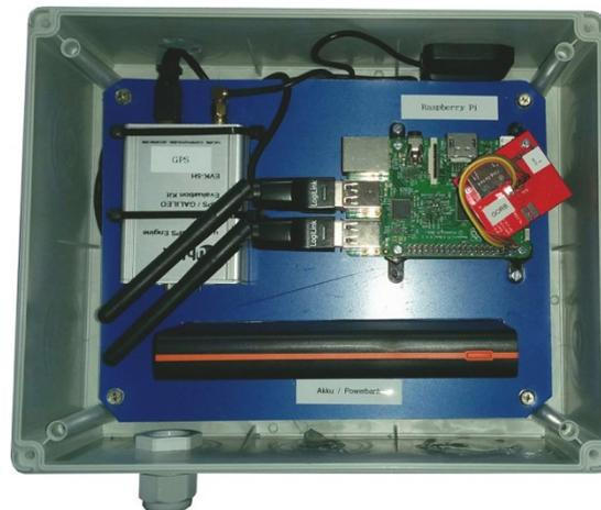
Figure 2: Mobile node on the field sprayer. It contains a GPS, a Raspberry Pi, a rechargeable battery for power supply and a connection for the temperature sensors attached to the sprayer's traverse.
