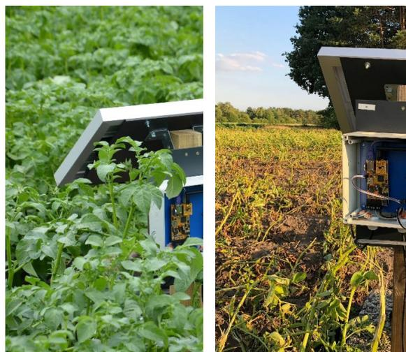
Figure 4: The figures show two different environmental conditions for the collecting nodes on the field. In the first picture the node is almost enclosed by leaves of the potatoes, in the second one the node is standing freely in the field.
