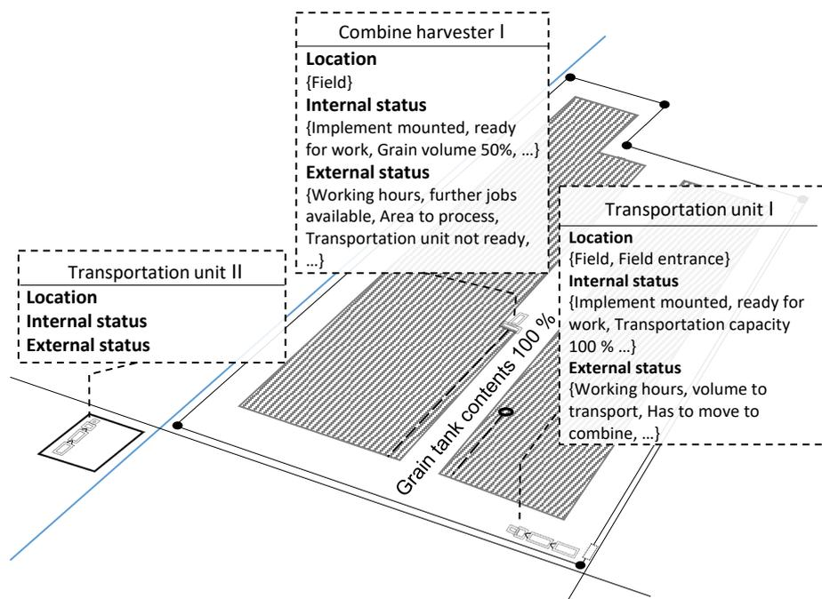
Figure 4: Process simulation on the example of transport during combine harvesting
