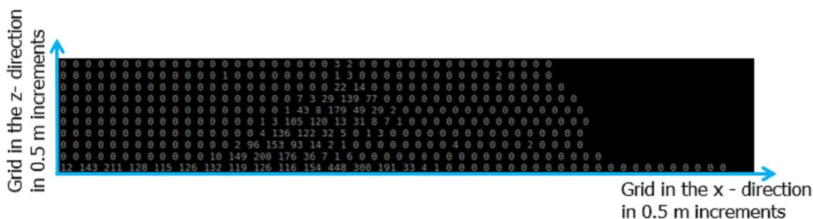
Figure 10: Representation of the radar points in the occupancy grid (© ZF Friedrichshafen AG)
