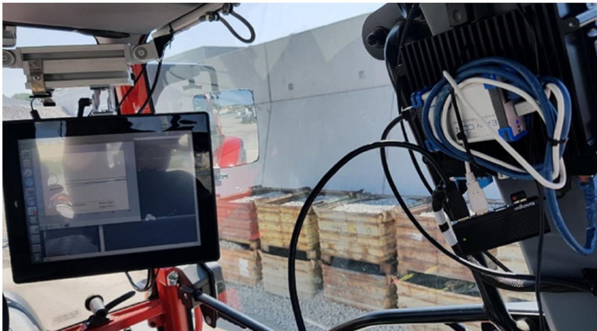
Figure 2: Installation of the system in agricultural machinery: HPC with display showing uphill gradient recognition (© ZF Friedrichshafen AG)
