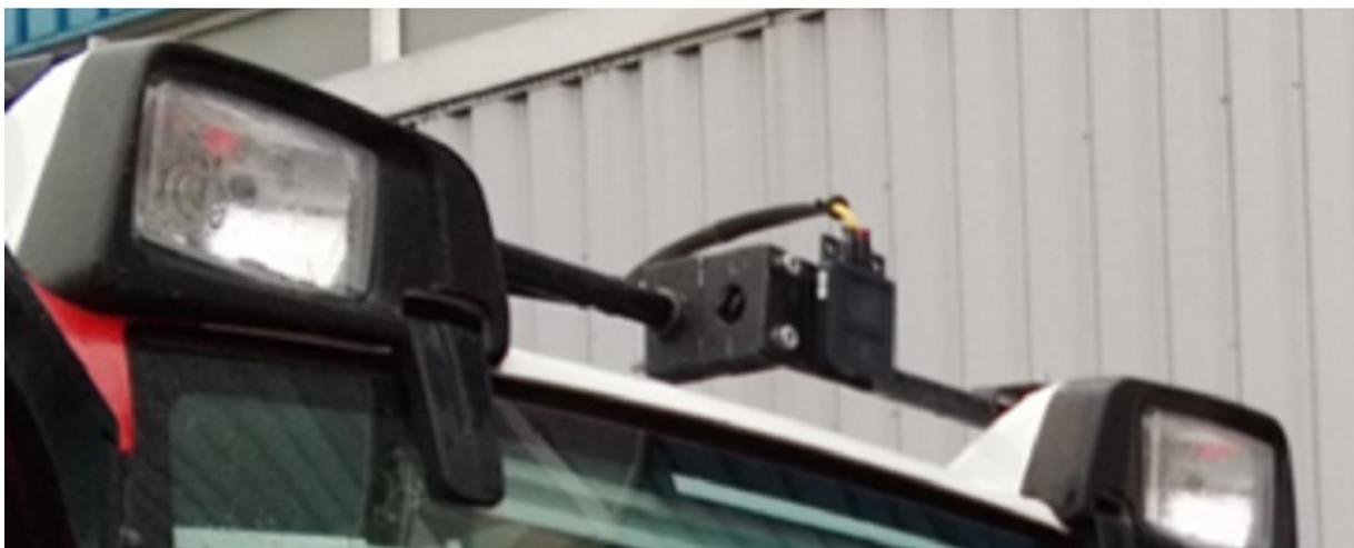
Figure 1: Radar mounted on agricultural machinery (© ZF Friedrichshafen AG)
