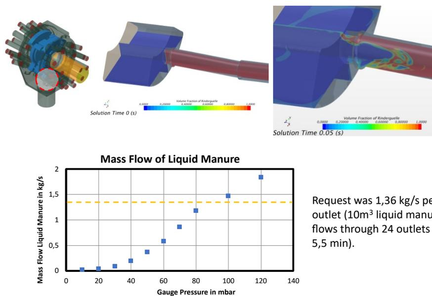
Figure 10: Minimum air pressure or volume flow to maintain the required liquid manure mass flow rate (© Riedel)
