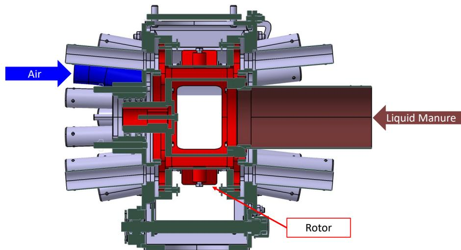
Figure 2: Sectional view of the executed liquid manure distributor (© Riedel)
