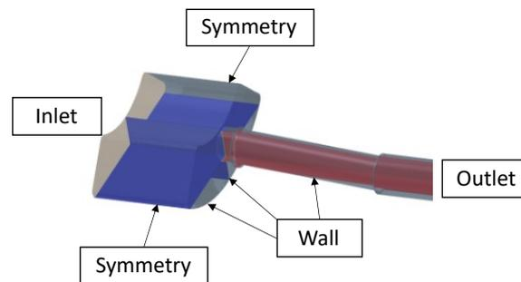
Figure 8: Boundary conditions on the CFD-model (© Riedel)
