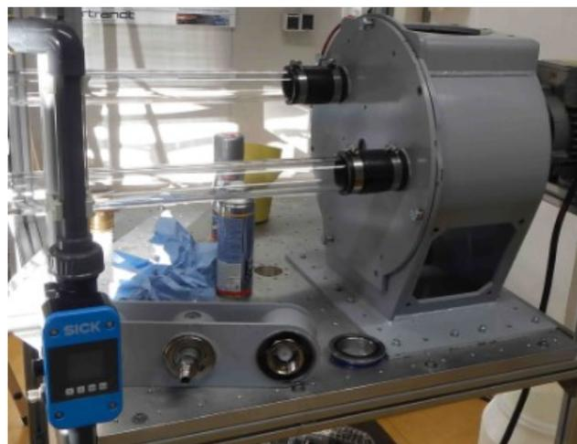
Figure 4: Test stand construction (rotor and acrylic glass panels still dismantled) (© Riedel)
