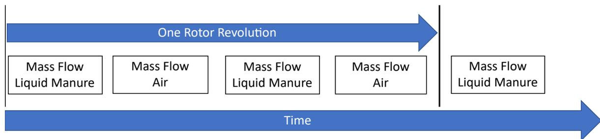
Figure 9: Cyclic inlet boundary condition to map rotor rotation (© Riedel)
