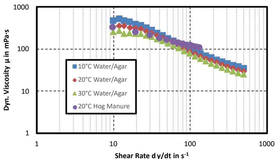
Figure 1: Dyn. viscosity vs. shear rate for a mixture of 1.2 % agar and 98.8 % water and in comparison, hog manure (TÜRK 1986)
