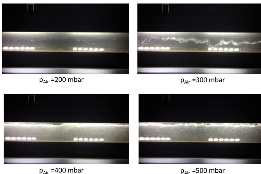
Figure 6: Influence of pulsating air on flow conditions in the outlet (water  $Q=70$  ltr/min) (© Riedel)
