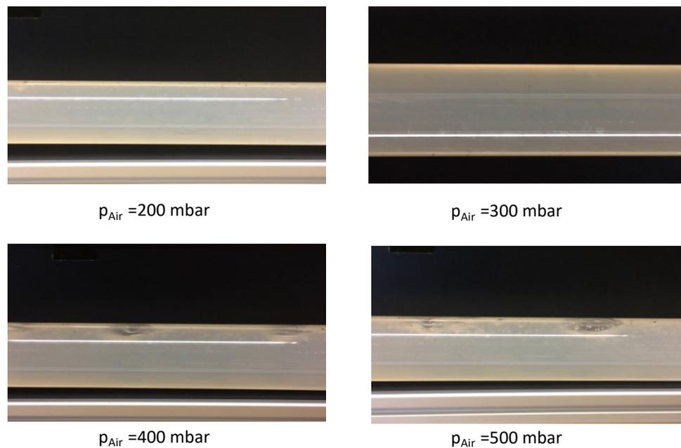
Figure 7: Influence of pulsating air on flow conditions in the outlet (water-agar $Q=70$  ltr/min) (© Riedel)
