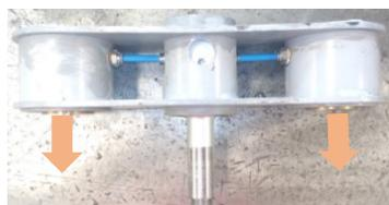
Spring loaded pressure piece to seal the distributor against the outlet (in the hollow shaft)
