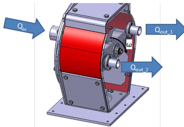
Figure 3: CAD representation of the test bench distributor, the side wall on the outlet side is shown transparent for display reasons (© Riedel)
