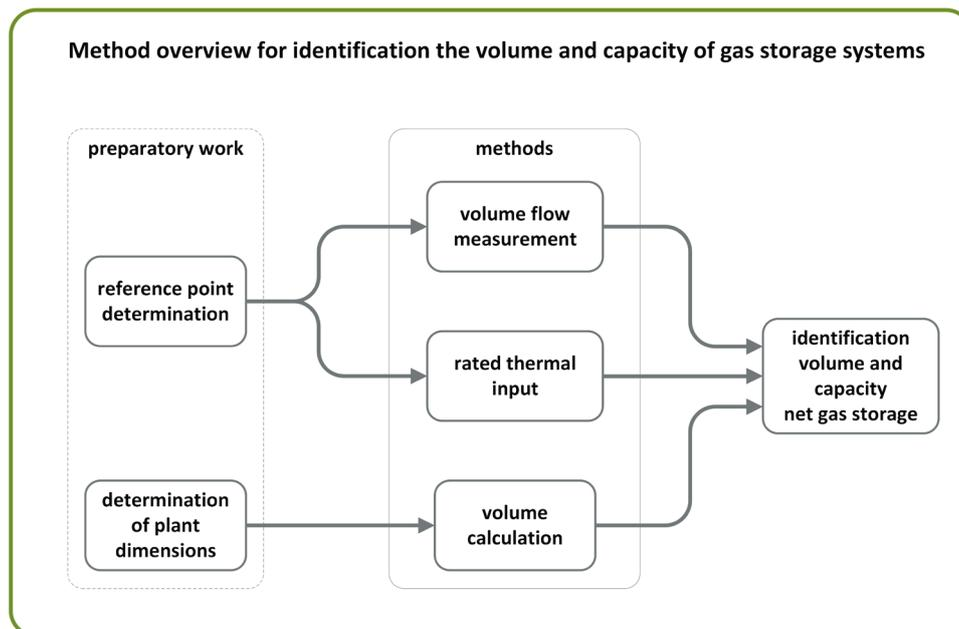
Figure 6: Overview of three methods to determine gas storage capacity and volume
