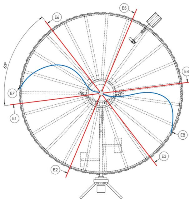
Figure 5: Top view of the gas storage roof; E1 to E6 position/route of the individual rope pulls of the rope pull measurement system in red; E7 and E8 position/route of the flexible tubes of both hydrostatic pressure measurement systems in blue
