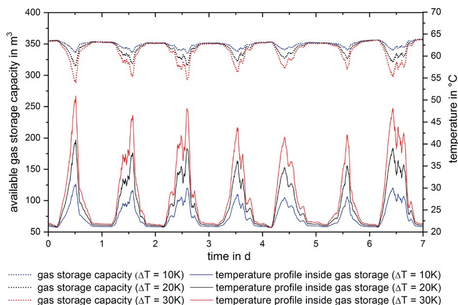
Figure 10: Mathematical illustration of the influence of the internal gas storage temperature on the available gas storage volume at different temperature spreads
