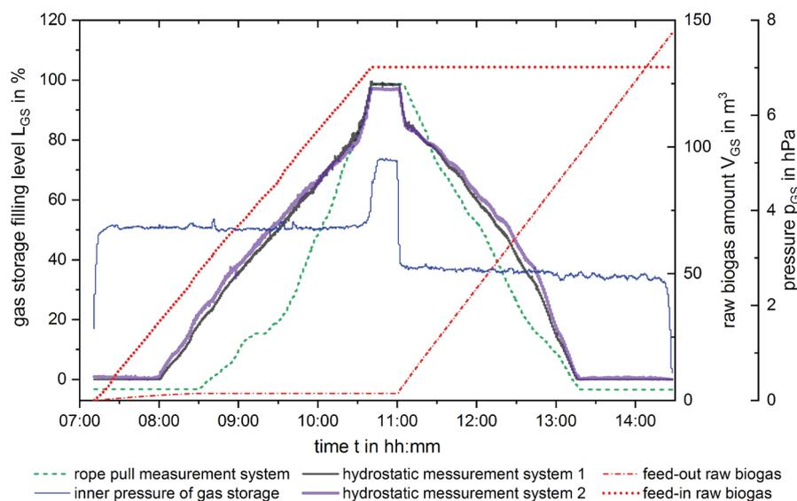
Figure 8: Representation of the characteristic curve of the integrated double-shell pneumatically preloaded membrane gas storage of the fermentation tank
