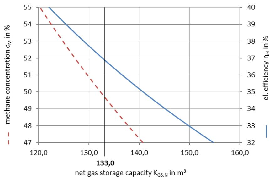
Figure 7: Representation of the range of the determined net gas storage capacity depending on an assumed methane content  $c_M$  of 49.7 Vol.-% and electrical efficiency  $\eta_{el}$  of 36.9% of the RBP-CHP unit; change in the net gas storage capacity with varying methane content (red dashed line) or varying efficiency (blue)
