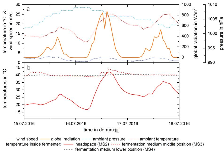
Figure 9: Influence of weather conditions on the course of temperatures in the gas storage and fermentation medium
