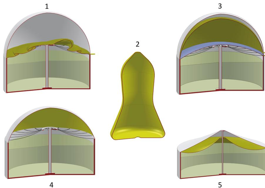
Figure 1: Selected designs of gas storage systems; 1 - integrated pneumatically preloaded double-shell membrane gas storage (partially filled); 2 - membrane gas bag suspended (partially filled, without supporting structure and enclosure); 3 - integrated pneumatically preloaded three-shell membrane gas bag (fully filled); 4 - gas pressure-supported single-shell membrane gas bag (fully filled); 5 - mechanically preloaded double-shell membrane gas bag (deflated)
