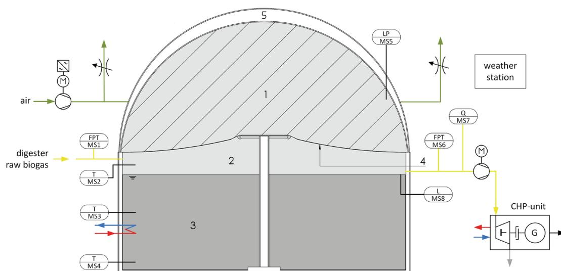
Figure 4: Representation of different gas storage areas in the technically full state; 1 - variable net gas storage volume (light grey hatched); 2 - variable gross gas storage volume (light grey and light grey hatched); 3 - fermentation medium volume (dark grey); 4 - belt support system; 5 - variable support air volume (white); legend measurement technique - F volume flow, L filling level, MS measuring point, P pressure, Q gas concentration and T temperature; weather station (Table2)
