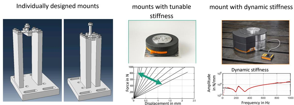
Figure 3 : Several options for simulating attachment stiffnesses. From the left: Individually designed mounts, mounts with tunable stiffness (MILLITZER 2021, HANSMANN 2018), mounts with dynamic stiffness (MILLITZER 2021)
