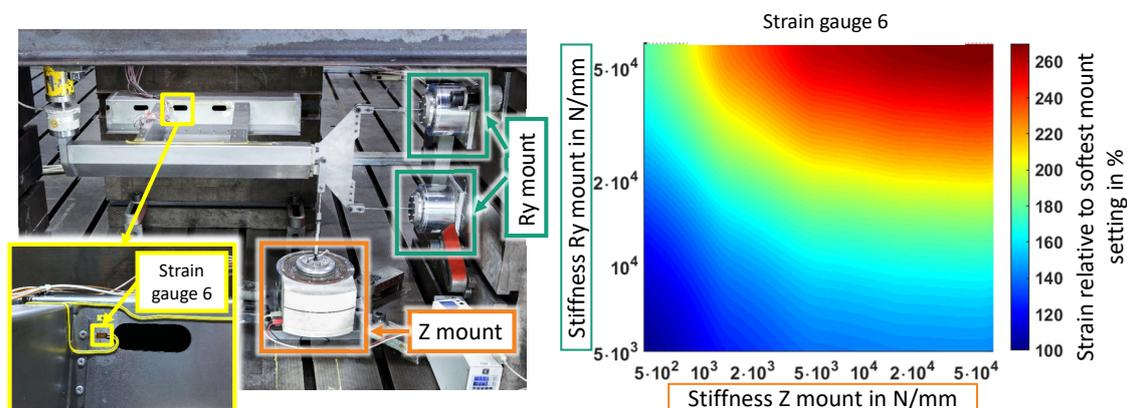
Figure 8 : Simplified equivalent test for a support structure of a structurally integrated high-voltage storage system (left) and dependence of the local strain on a selected strain gauge on the stiffness of the tunable mounts (Z and Ry mounts) in this test setup (right) (LANDERSHEIM et al. 2022)
