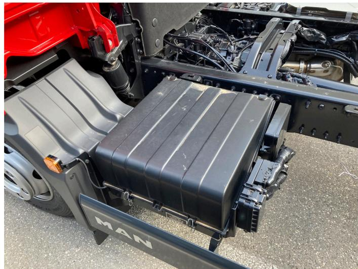
Figure 4 : Battery box attached to the frame of a 12t-class light truck (© MAN)
