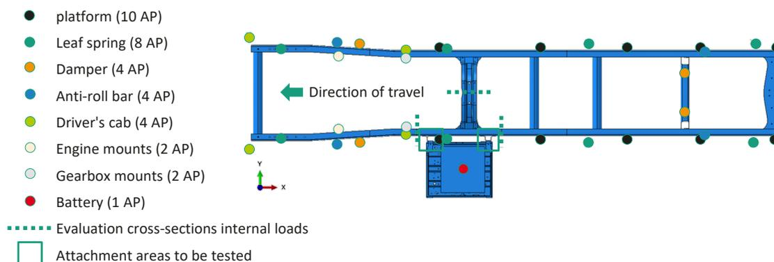
Figure 5 : Load application points in the frame of the commercial vehicle (AP: attachment location) (LANDERSHEIM and KÜPPERS 2022)
