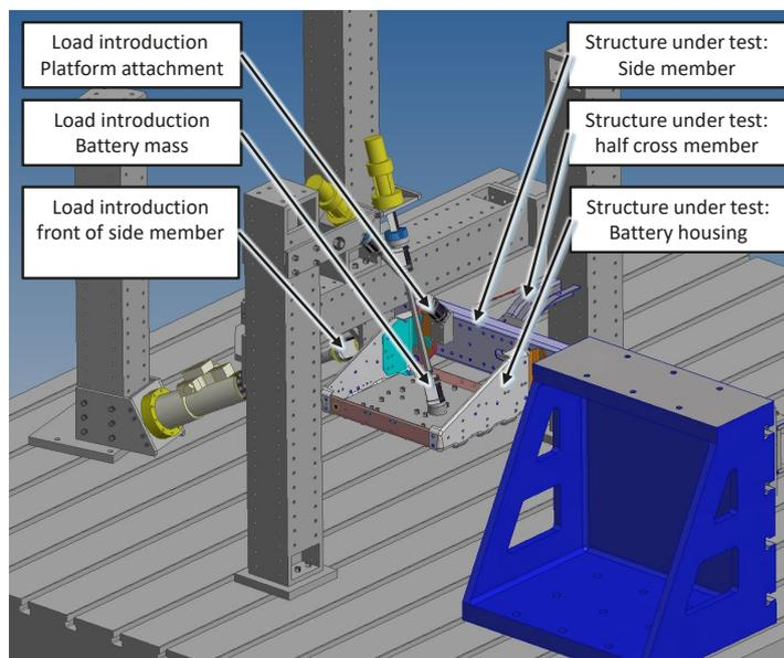
Figure 7 : Simplified replacement test designed for testing the battery attachment (Landersheim and KÜPPERS 2022)
