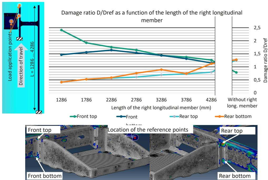
Figure 6 : Relationship between the damage at four reference points at the battery attachment and the clamping length of the opposite longitudinal member in relation to the reference damage (LANDERSHEIM and KÜPPERS 2022)
