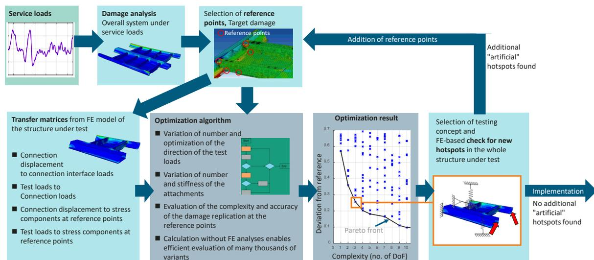
Figure 2 : Procedure for optimizing the substitute test
