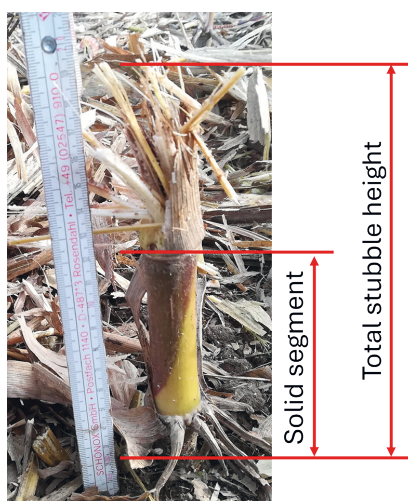
Figure 2: Corn stubble height measurement scheme (© S. Ramm)
